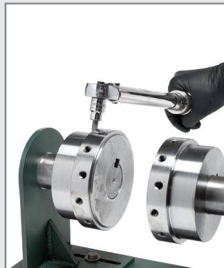
Step 1: Fasten shaft hubs
