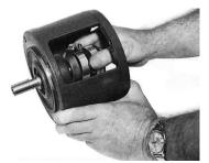
2. Insert Flexidyne unit thru the slots in the end of the module, knurled end first, and into rubber element.
