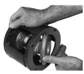
It is recommended that the reducer be firmly attached to its support before installing C-Flex module and motor. Stake C-Flex module output shaft key in position and insert module into reducer. Install and tighten bolts to 360 in-lbs.
