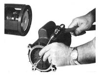
5. Slide motor shaft into Flexidyne unit. Install and tighten bolts. Locate rubber element so that it is flush with knurled end of C-Flex module output shaft. Locate clamp flush with end of rubber element and tighten clamp screw snugly.
