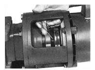
7. Remove the filler plug and install the proper amount of flow charge specified in Table 1. Replace and tighten filler plug, making sure that no flow charge is trapped in the threads. Torque filler plug screws to 35 inch-pounds. Where the C-Flex installation is exposed to operating personnel, it is advisable to use the mesh-type guard provided. Drill 2 holes in the module housing for self-tapping screws. Wrap guard around housing and secure with screws.
