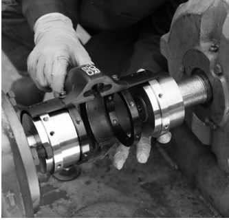
Figure 7 - Install Element Half with High-Speed Rings
