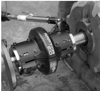
Figure 8 - Install Second Element Half on Hubs with High-Speed Rings
