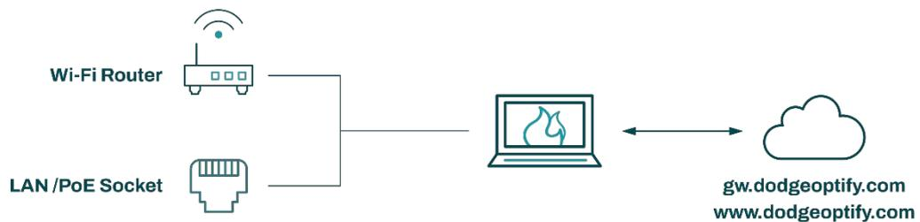
Figure 13: firewall configuration
