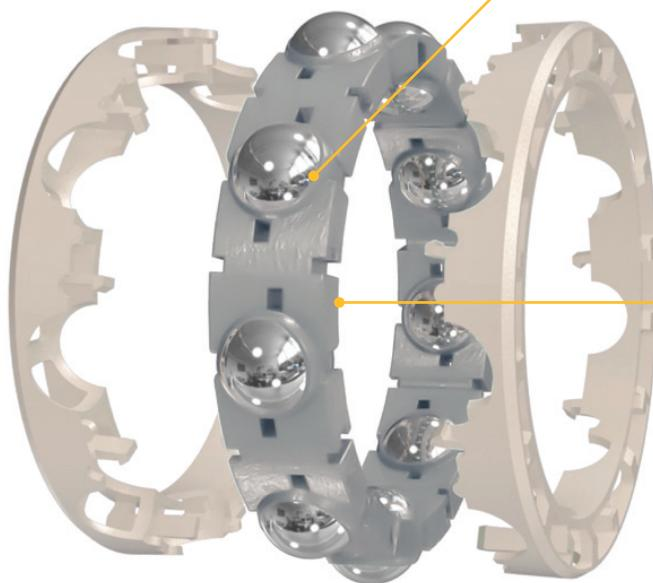
Unlike standard designs, the Maxlife cage holds a large volume of grease to ensure constant contact with rolling elements
