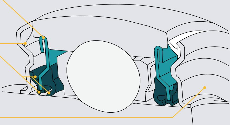
Stainless-steel flinger is extended for greater protection under high-pressure washdown
