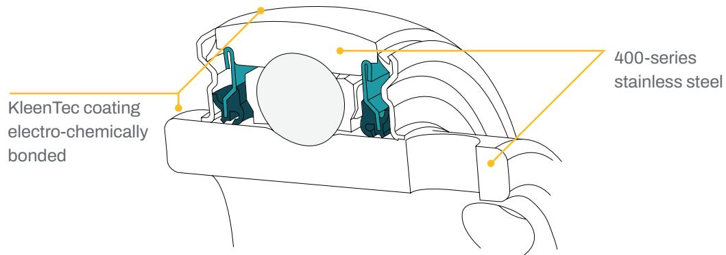
Processing equipment, which commonly includes ball bearings, is frequently washed with high-pressure water and chemicals to maintain a clean, hygienic production environment. This type of environment is extremely tough on bearings.
