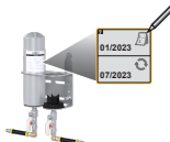
For remote mounting: note the activation date on the label
