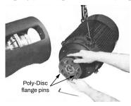
Mount C-face motor to C-Flex module and tighten bolts. Inspect spring between coupling flanges to ensure that the Poly-Disc element spacer buttons press lightly against coupling flange faces. (Refer to steps).
