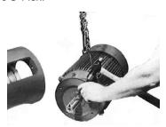
5. Loosely assemble Taper-Lock bushing into Poly-Disc® flange and fit onto motor shaft (pins extending away from motor). Position flange such that motor shaft is recessed 1/4" for the model 500 and 3/16 for the model 1000. Tighten bushing securely into place according to the instruction manual supplied with bushing. When assembled (step 6), the spacing should cause the Poly-Disc element spacer buttons to lightly press against the coupling flange faces.
