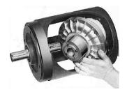
It is recommended that the reducer be firmly attached to its support before installing C-Flex module and motor. Stake C-Flex module output shaft key in position. Insert C-Flex module on reducer shaft. Tighten bolts to 900 in. lbs.
