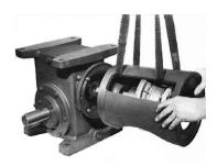
Stake motor shaft key in position flush with end of motor shaft for the 500 C-Flex and 9/16" from end of motor shaft for the 1000 C-Flex.
