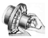
Insert Flexidyne mechanism through the large access hole
