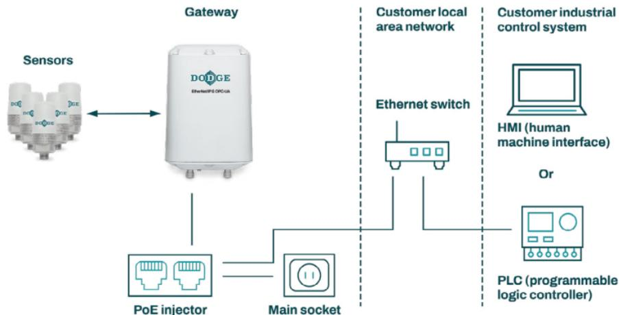
**Figure 5 - LAN network configuration**
