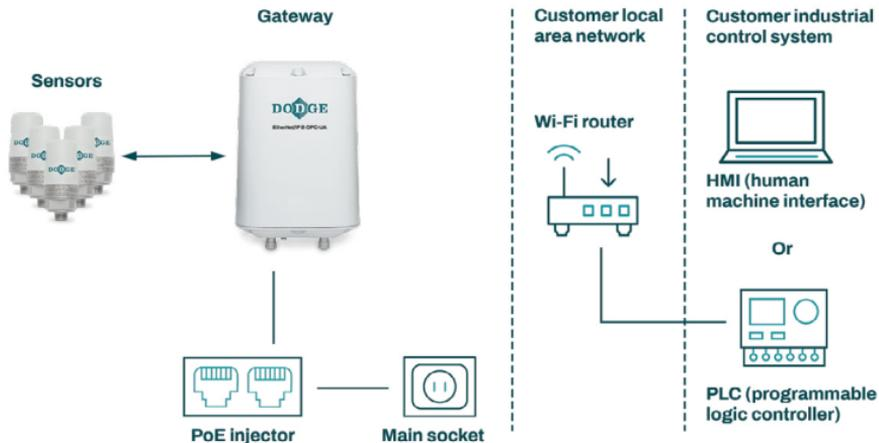
**Figure 7 - Wi-Fi network configuration**
