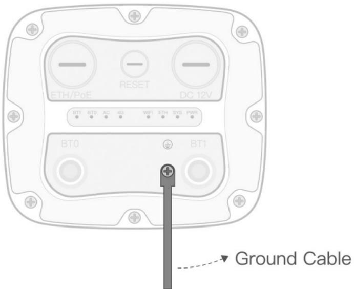
**Figure 2 - Grounding cable location**
