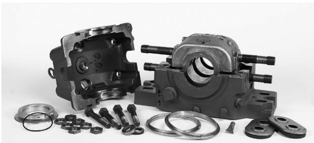
Exploded view of expansion pillow block (housing cap and liner cap not shown). Non-expansion pillow block includes thrust plate kit and split thrust collar.
