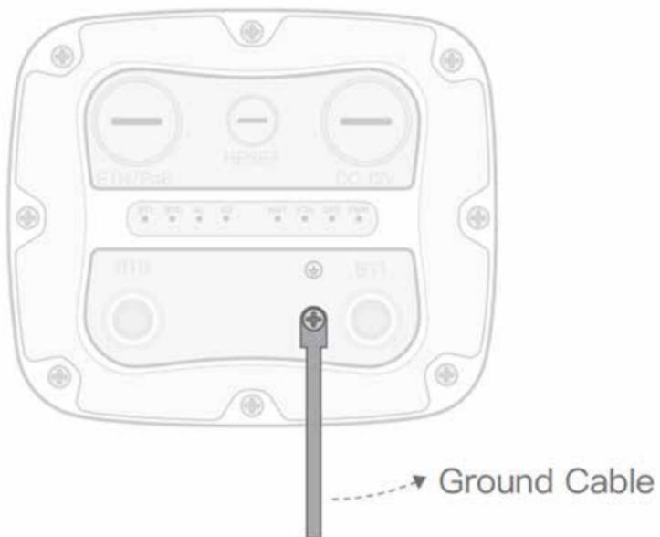
**Figure 2 - Grounding cable location**
