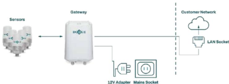
**Figure 11 - Wi-Fi network configuration with 12 V adapter**
