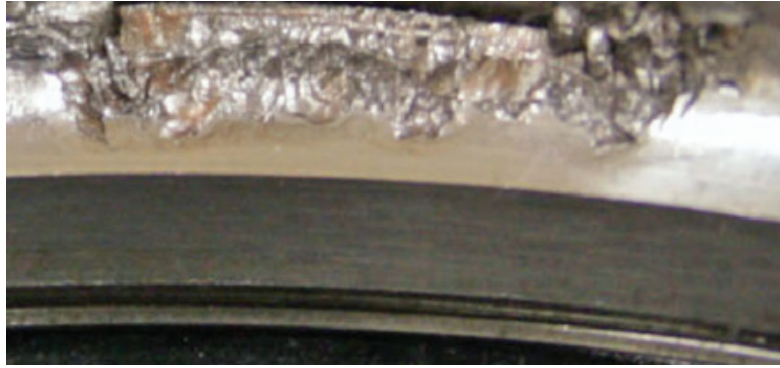
Figure 18 - Bearing lubrication failure
