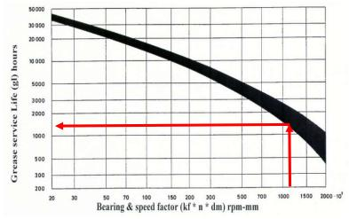
Using the Grease Service Life (gl), determined from the above diagram, the Re-lubrication Interval can now be calculated. Depending on the operating conditions there are two ways to calculate the Re-lubrication Interval. If the operating and environmental conditions are favorable use the equation in Case #1. If operating and environmental conditions are poor, then reduction factors (f1,
