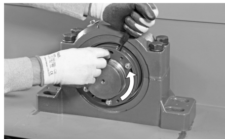
Figure 4 - Holding external nut and rotating internal nut using hex head bolt
