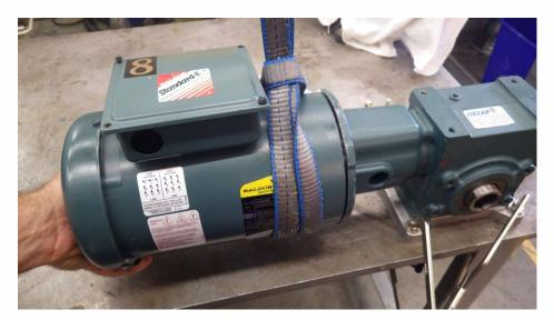
Slowly rotate the motor to the desired conduit box position. The lifting strap / straps may
